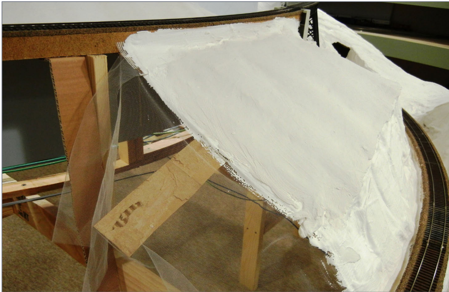
6. Using tulle over the cardboard strips as a “screen mesh” to hold up the plaster scenery.
