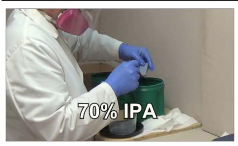
8. Once de-plated, the parts are cleaned with isopropyl alcohol (IPA). John starts with 90% IPA, and then rinses the part with 70% IPA. He uses used airtight coffee containers to both store the IPA and bathe the parts. He then allows the parts to dry for up to 24 hours on paper towels.
