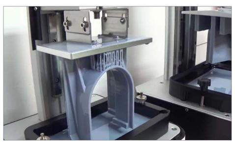
6. Multiple resin 3D-printed tunnel portals hang off the build plate after printing. Some of the prints took 9 hours to complete.
