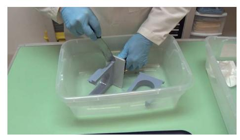
7. A putty knife with a sharpened edge is used to remove the prints from the build plate. The knife is kept as flat as possible to slide under the print.
