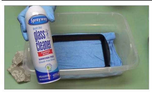
4. John demonstrates how to clean and prepare the resin tank from the 3D printer prior to beginning printing.
