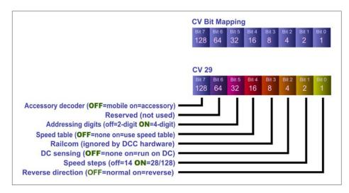
5. CV bit mapping as shown here on the shortcuts card lets you compute the specific decimal value to put into a CV. See the text for details.
