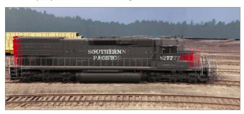
4. When programming a loco on the main, most decoders acknowledge receiving a value by jumping the loco ahead slightly. If you don't see this "jitter" when programming on the main (POM), the loco may have dirty wheels, be sitting on dirty track, or both. Try sliding the loco back and forth and then sending the POM command again to see if the loco now responds with this characteristic jitter.
