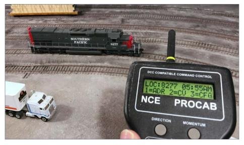
3. When the DCC shortcuts card recommends setting decoder CV values directly, we're talking about using the CV programming on the main feature of your DCC system. Here I'm using my NCE Procab hammerhead to program loco 8277 on the main. My next step will be to press the 2 button for programming CVs.
