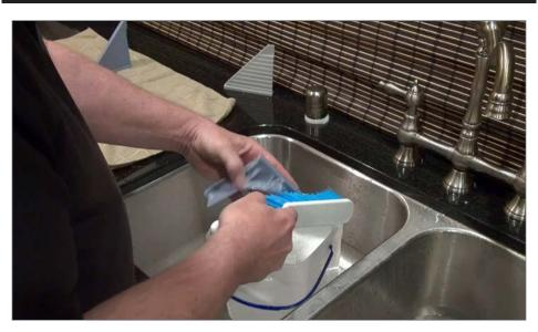
10. The models are then washed in laundry detergent and water, rinsed with clean water, and left to dry.
