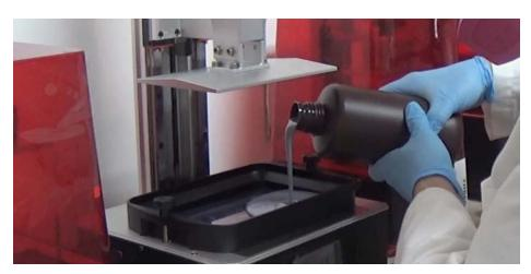
5. After shaking the resin in the bottle to ensure it is completely mixed, John pours it into the tank. Bubbles formed by shaking will rise to the surface by leaving the resin to sit for about 15-30 minutes. The bubbles can be soaked up with a towel or moved to the edge with a scraper.
