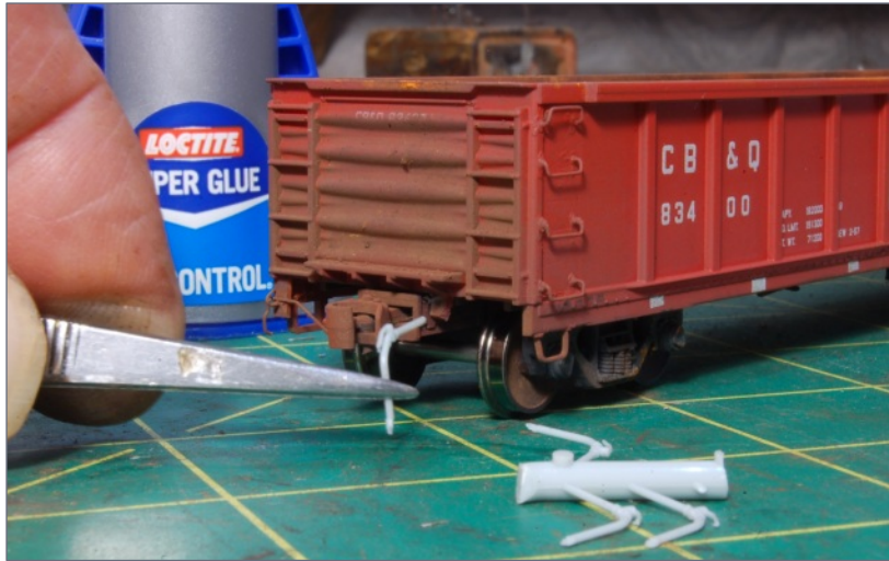
19. My favorite air hose is Detail Associates number 6206. A true scale air hose model for sure.
