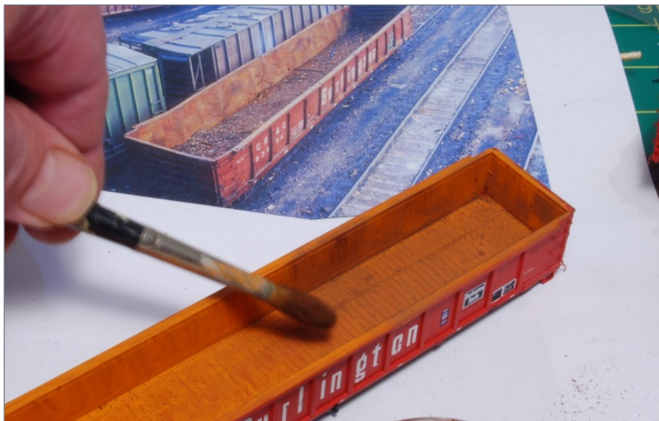
15. When the paint was dry, I applied dark weathering powders.
