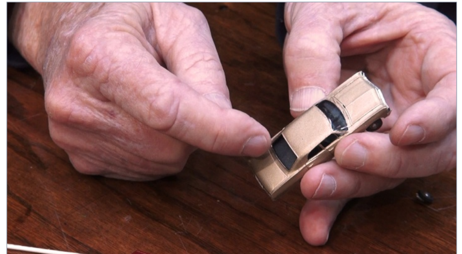
19. Mike describes how his friend John Tyson scuffs the edges of the window openings with fine sandpaper to avoid having paint pull up when the modeler peels the tape off the edges.
