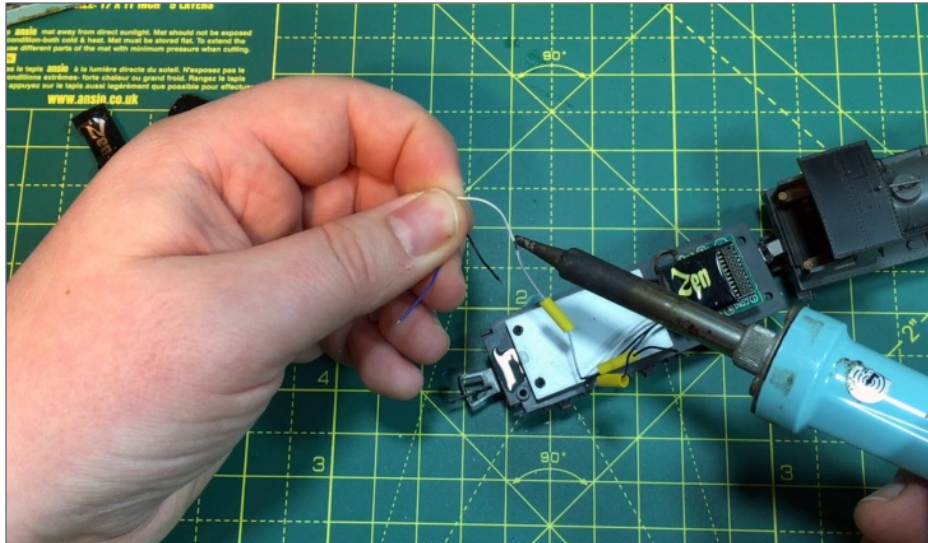
4. Jenny shows how to strip, tin, and solder wires together.
