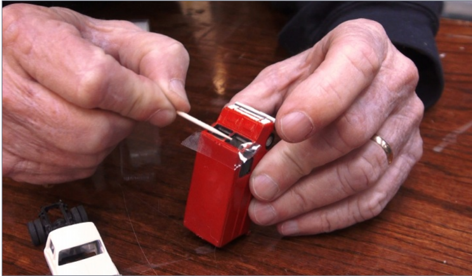
12. After laying the tape across the windshield opening, Mike burnishes it into place with a toothpick.
