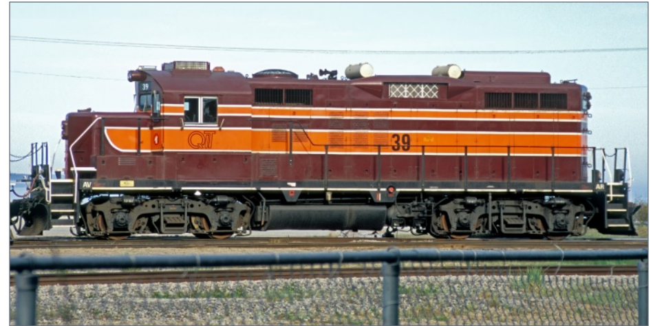
28. QIT purchased GP9 39 from Quebec Cartier Railway in 1987. The Pointe St. Charles shops in Montreal rebuilt it in the early 1990s to the same standards as CN's rebuilt GP9s.
