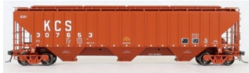
PS-2CD 4750 cu. ft. triple-bay covered hopper car.
