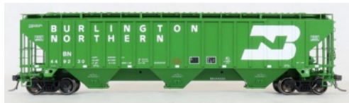
PS-2CD 4750 cu. ft. triple-bay covered hopper car.
