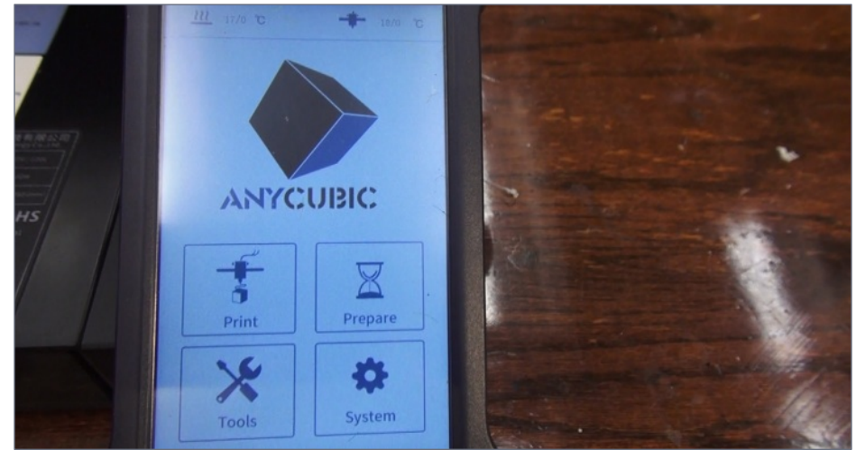
14. An LCD screen is used to control the printer, from auto-leveling the bed to selecting the file to print.
