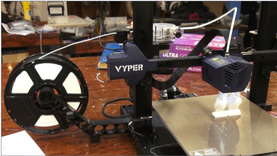
16. The printer feeds the filament off a spool and into the printhead, where it is heated up to 500° Fahrenheit (260° Celsius) before being deposited onto the print.
