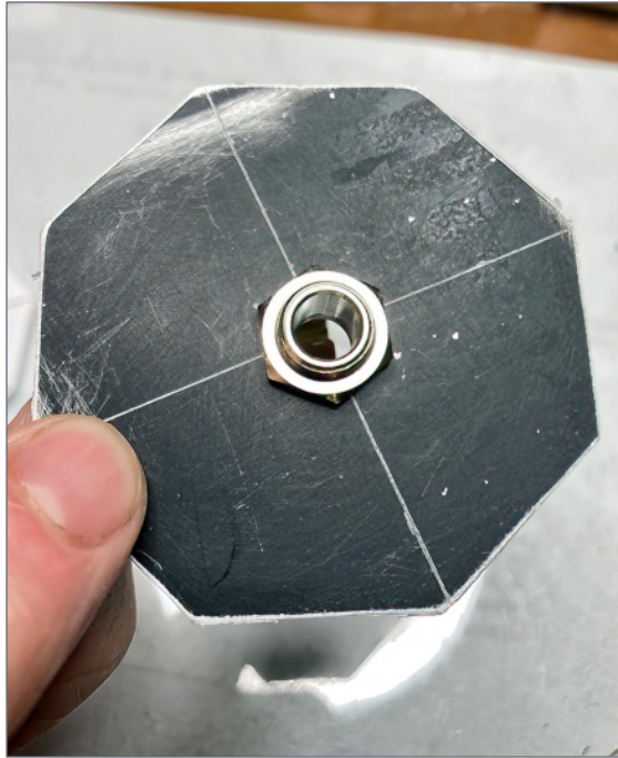
15. I marked the center, then I used a succession of drills to make a hole to mount the jack.
