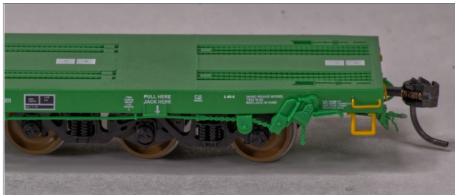
5. The FGE car features the Wabtec Model 9020 hand brake lever.
