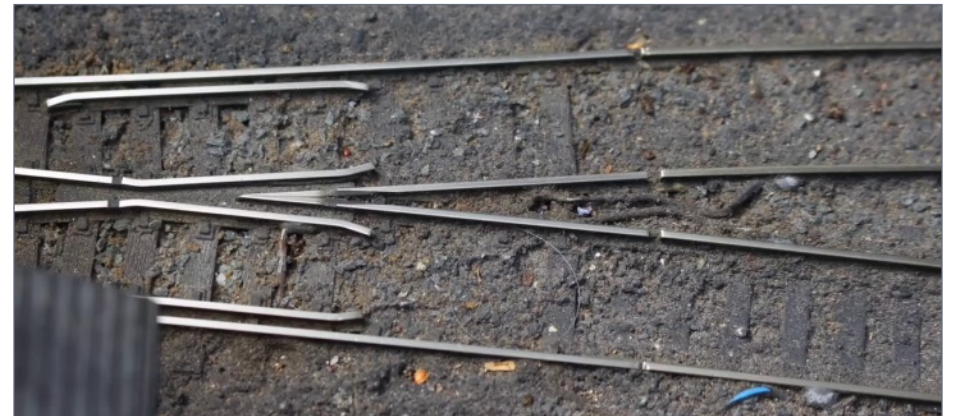
3. To deal with expansion and contraction, each section of track has a 1mm gap between it and the next section. Trevor hasn't had any temperature-related rail issues, although it does get up to 100°F in the summer.
