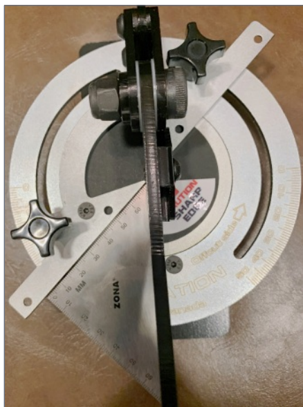
11. Testing the 45-degree angle with my Zona Triangle.
