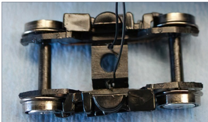
5. Truck hole positions with electrical wire pickups shown.
