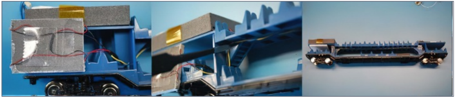
38. Lower-level front/rear lighting fixture installation and wire routing.
