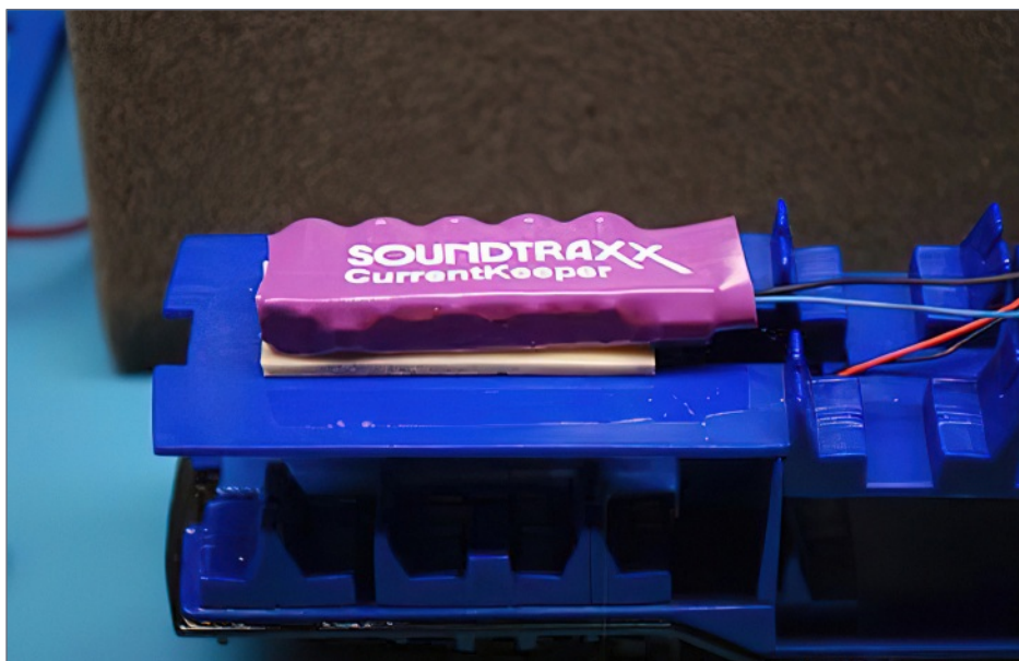
18. Current Keeper wire extension and placement.
