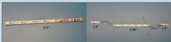
42. ESU boards, cut and wired.
