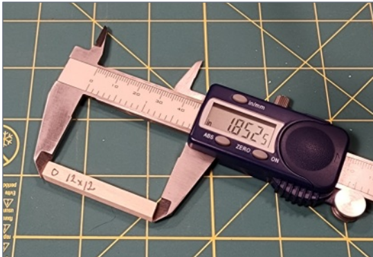
15. Measuring the cuts using a digital caliper.
