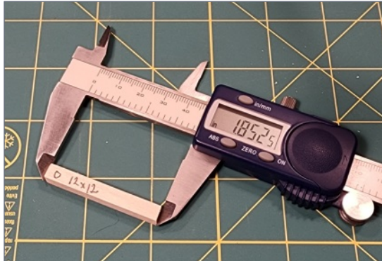
15. Measuring the cuts using a digital caliper.
