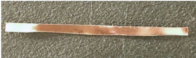
7. Phosphor-bronze pickup wiper; cut four of them.
