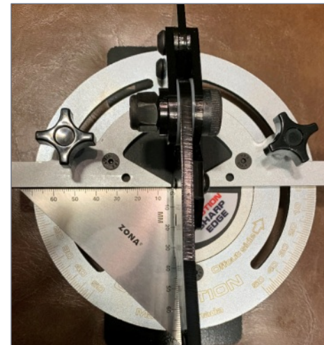
10. Testing the 90-degree alignment with my Zona Triangle.
