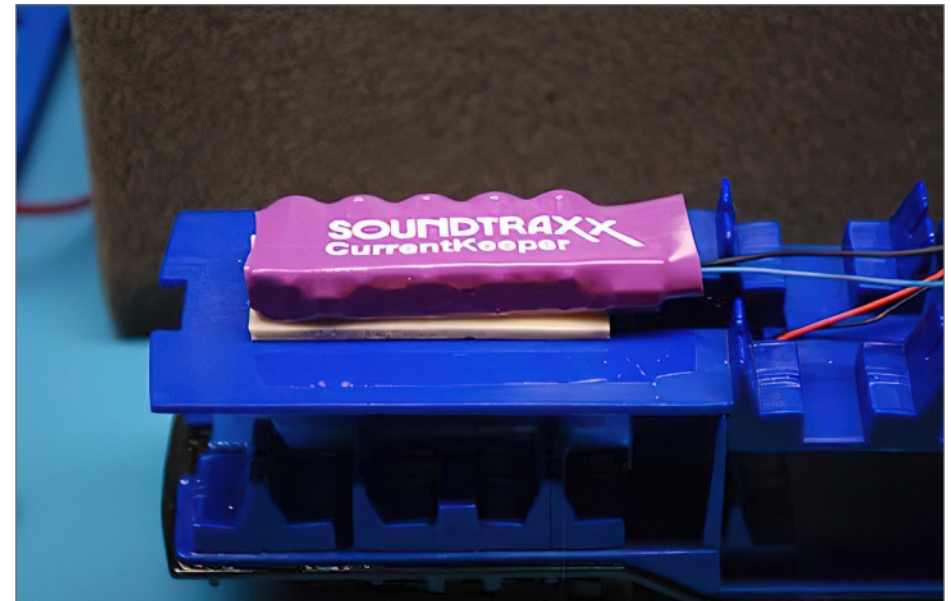
18. Current Keeper wire extension and placement.
