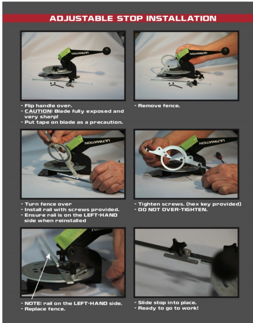
6. Ultimatum instructions for installing the repeater arm.
