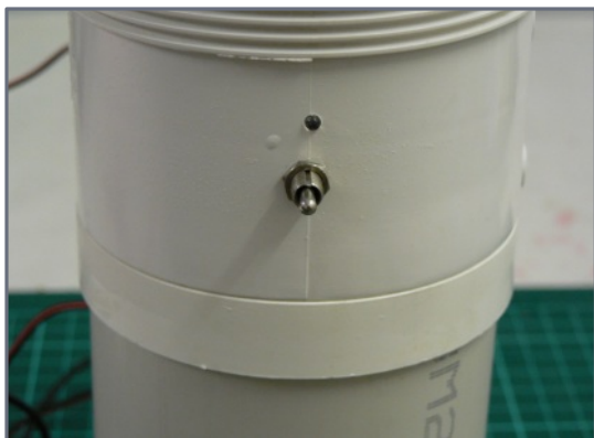
9. The switch and LED in place.
