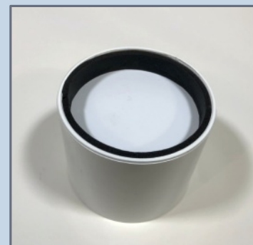
1c. On the other end of the coupling, I applied the full 5/8" width weatherstripping around the inner lip of the coupling. Then I used styrene cement to glue the 0.060" styrene baffle disk I had cut. I applied the cement along the edges on both sides of the baffle and let it set up for a couple of hours.
