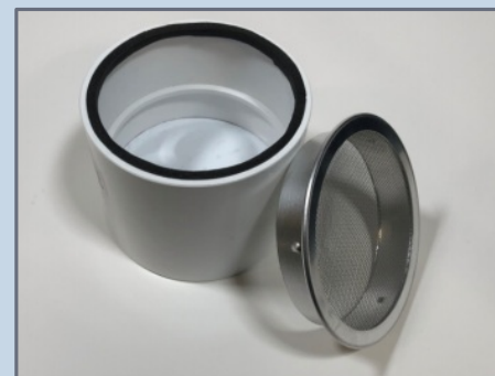
1b. I cut a 1/8"-wide piece of weatherstripping about 12.5" long and applied it around the inside lip of the coupling on one end. This made for a tight press-fit for the screen cover into the opening, with the metal bumps nestling behind the edge.
