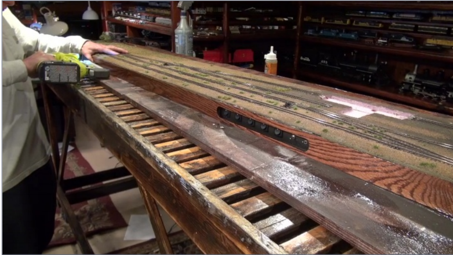
4. After the wood sections have dried, Ken glues the pre-stained plywood frame on, securing them with crown staples.
