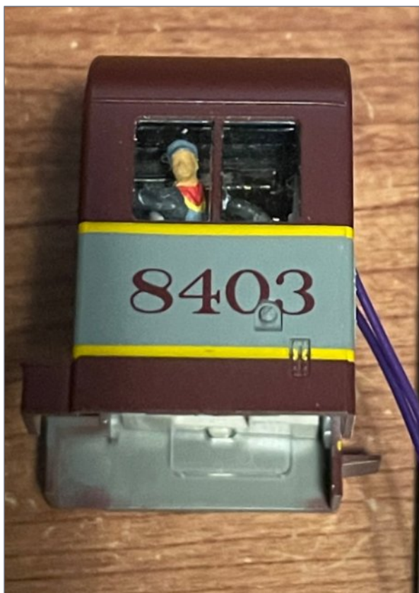
13. Cab insert and finished speaker (with black enclosure) installed into the cab.
