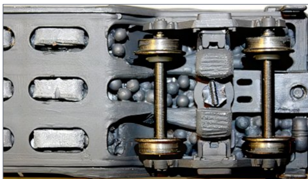
6. Weight in frame cavities and on truck.
