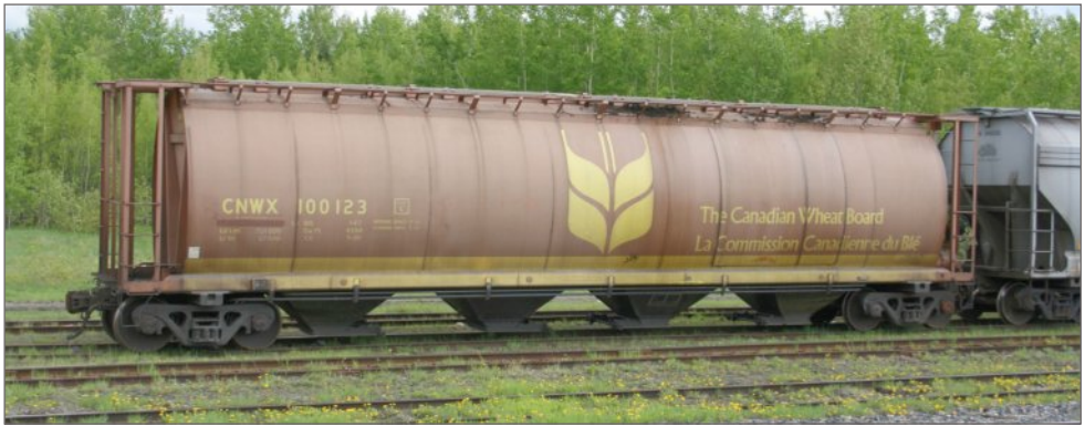
1. Example of the Marine Industries 4550-cuft cylindrical hopper.
