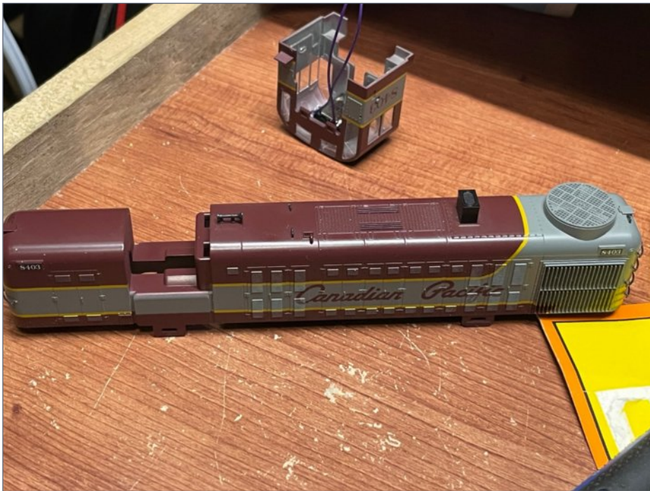
14. Look into the cab and you can see the black speaker enclosure assembled and attached to the cab roof.
