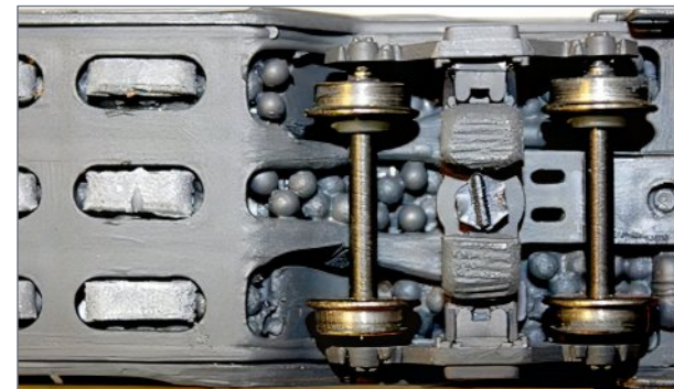
6. Weight in frame cavities and on truck.
