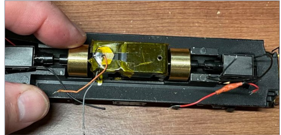
18. I broke a red truck wire while inspecting the gear box lubrication during current testing, so I needed to remove and disassemble the trucks. The gear tower covers need to be removed to access the trucks for disassembly.
