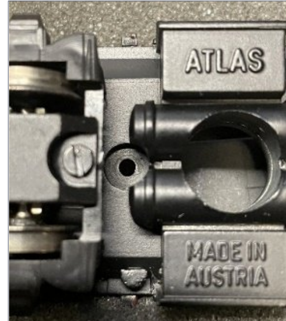
19. At center is the hole for the motor mounting screw.
