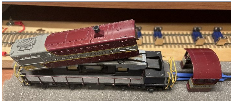
10. Tilting up the long shell.
