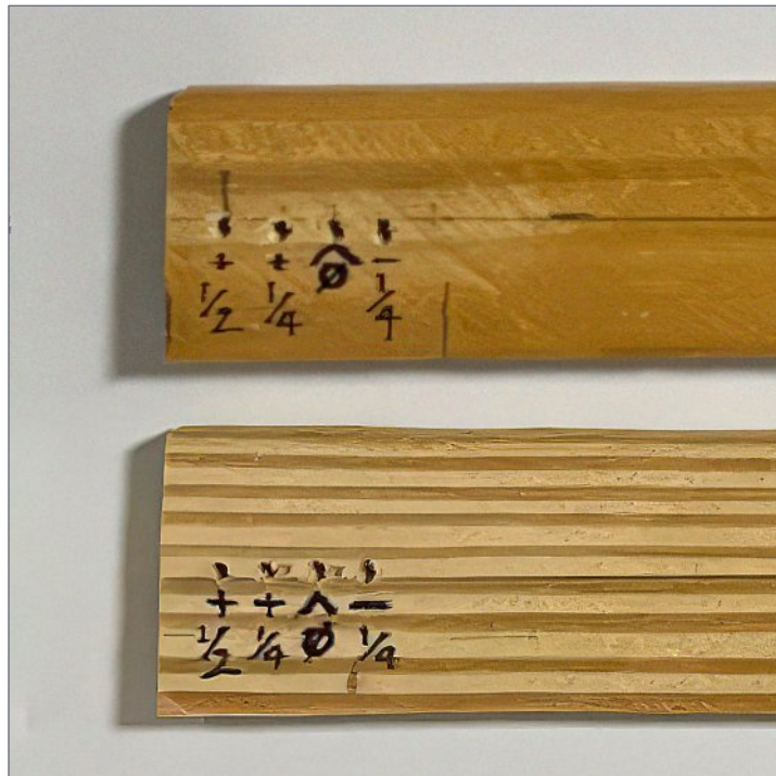
6. Closeup of the center-pin end of these curve-drawing sticks. Note the zero hole, as well as a -1/4" hole and +1/4" and +1/2" holes.
