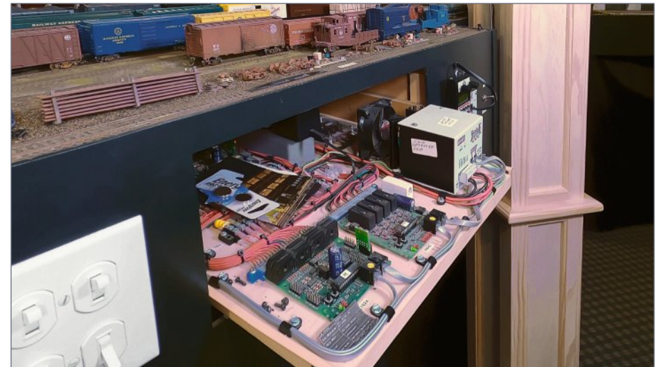
13. Each booster district on Jim's layout has a nice pull-out drawer with all the electronics placed neatly on it. This one is just below West Pittsburgh yard.
