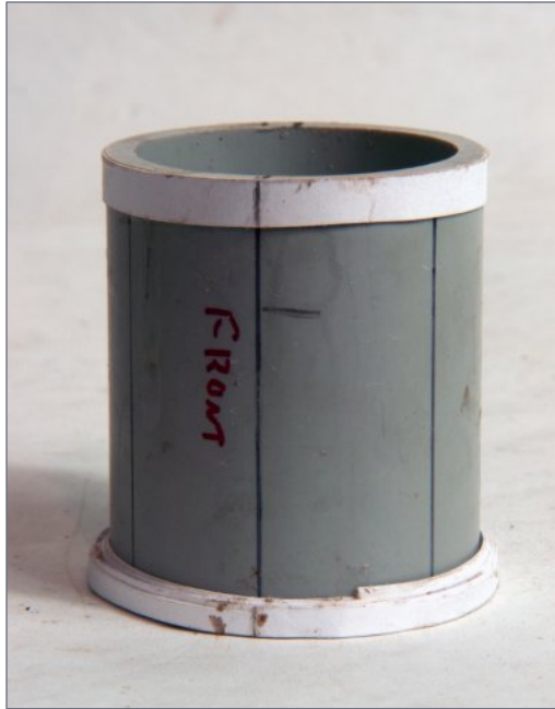
2. The pipe with the completed taper bands.
