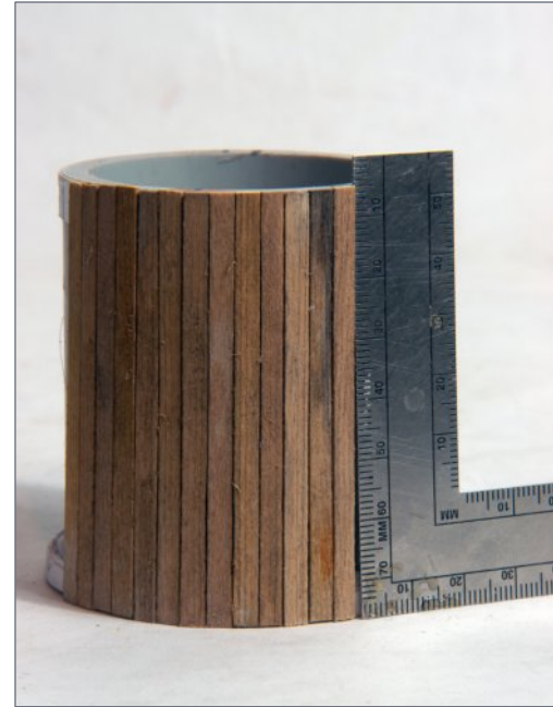
4. The error begins to show about halfway toward the back of the tank. The first stave is plumb, but the last stave is now noticeably out of plumb.
