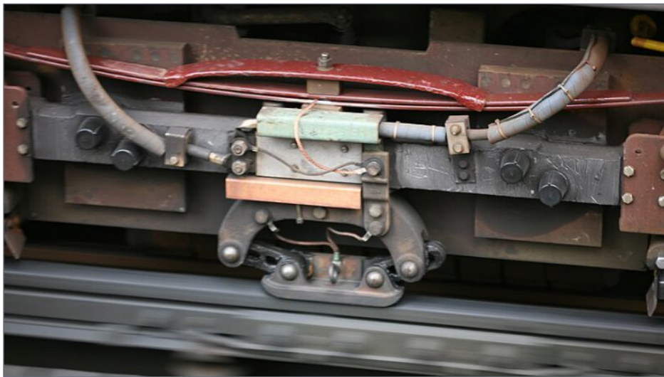
2. Overrunning pickup shoe on a Chicago L train. Wikimedia Commons image
