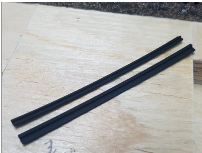
9. Painted 3D-printed “rubber” inserts.
