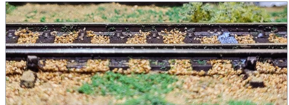
9. The third-rail is threaded through the chairs, and the nibs glued to the tie extensions.
