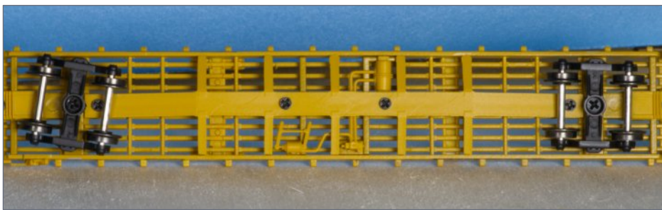
4. Underside of the N scale 60' Pullman Standard container car with brake components and lines.
