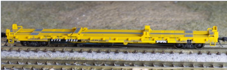
2. VTTX 91983 configured for a 40' and a 20' container.
