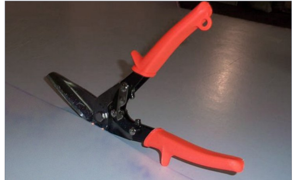
3. Tin snips with offset handles were perfect for cutting FRP.
