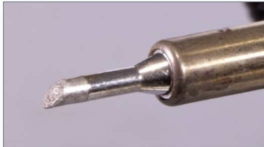
11. For soldering feeders, I like to use a bevel tip on my 60-watt soldering iron.
