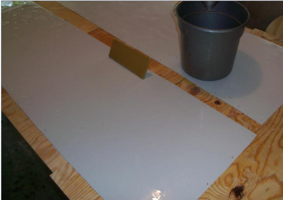
5. Materials ready for wet sanding, including the bucket of water that keeps dust down and improves results.
