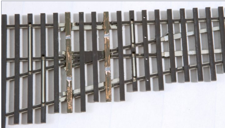
14. Note this older Walthers/Shinohara turnout already has jumpers between the stock rails and the closure rails, so I did not need to add them.
