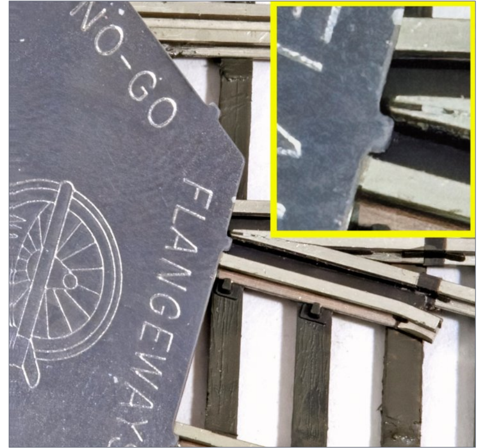
12. Here is how the NMRA gauge fits into the frog after correcting the guard rails. Notice in the enlarged view the gauge tab now easily clears the frog point. This guarantees the wheel flange will no longer pick the frog point. This now in-spec frog should give zero derailment performance with in-gauge wheelsets. Compare this to the gauge tab location in [11].
