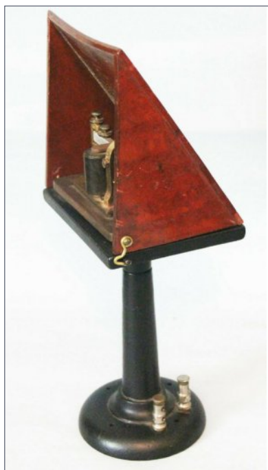
21. Sounder in resonator, side view.
