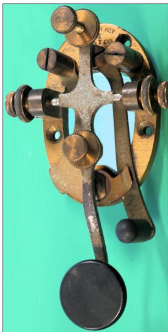
23. WE switch lever closed normal.
