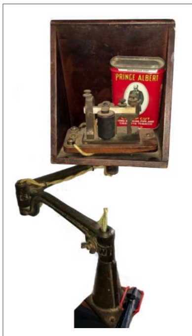
22. Western Electric telegraph sounder mounted in resonator.
