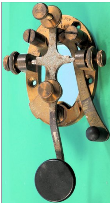
24. WE switch lever open, ready to transmit.
