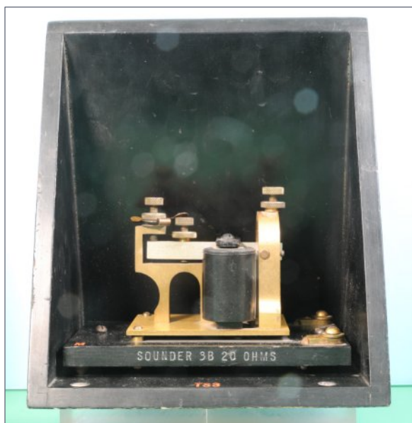
20. Telegraph sounder in a resonator box.
