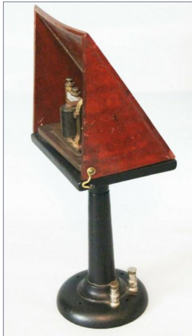
21. Sounder in resonator, side view.
