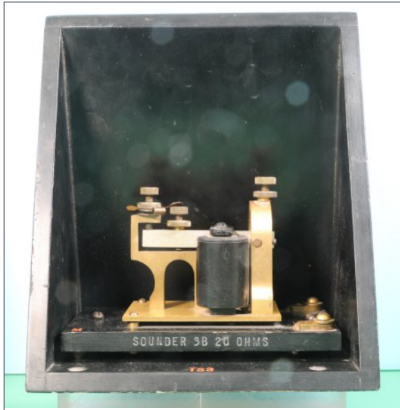
20. Telegraph sounder in a resonator box.
