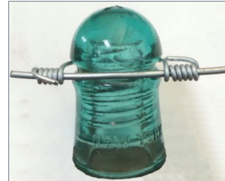
12. A wire tied to an insulator, similar to the diagram in [11].
