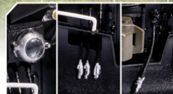
DITCH LIGHTS MU RECEPTACLES TRAINLINE HOSES
