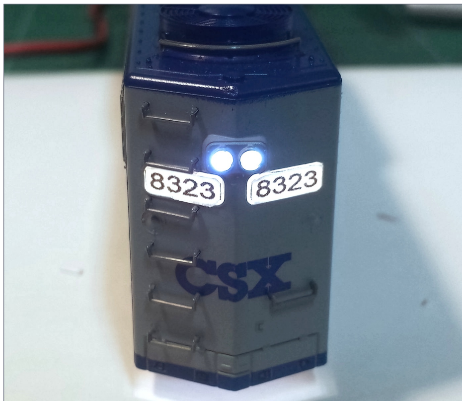
18. The completed rear hood with the LED headlights and number boards showing zero light bleed through the hood.
