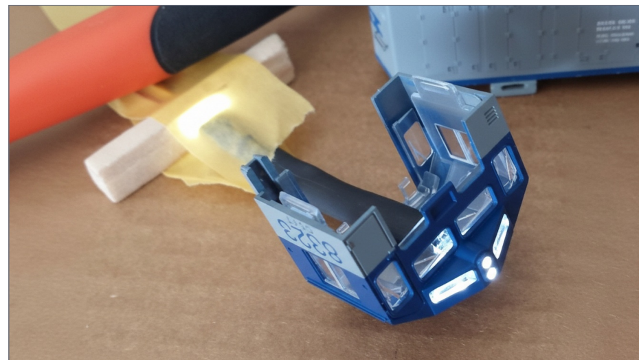
12. Cab light tube wrapped in shrink tubing and test-lit on the bench to check brightness, and to plan the final lighting solution.
