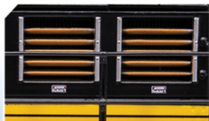
DYNAMIC BRAKE CAB (FIREMAN'S SIDE)
