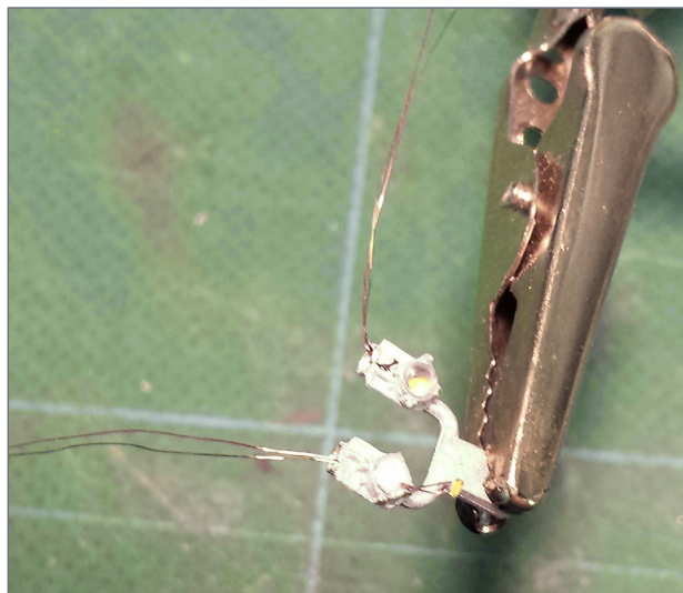
33. Lower LED with Krystal Kleer added to form a lens. Upper light has dried already.
