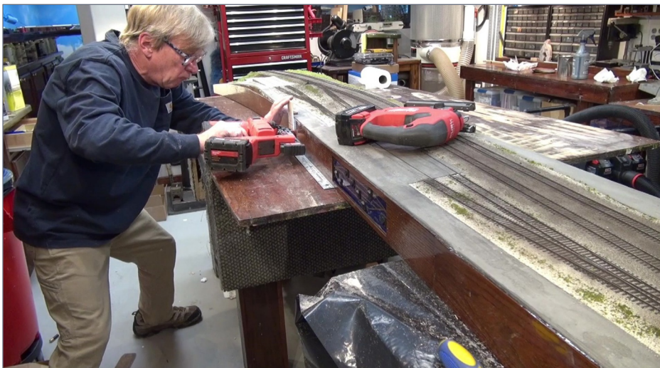
11. After carefully cutting the hole for the control panel, Ken glues and staples the fascia boards onto the module.
