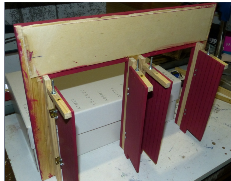
6. Screws used to connect the doors to the servos.
