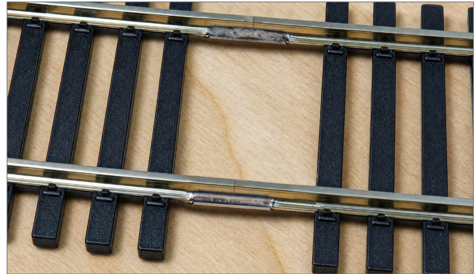
6. The lower rail joiner solder joint is good, but the upper one is a cold solder joint and needs to be redone.
