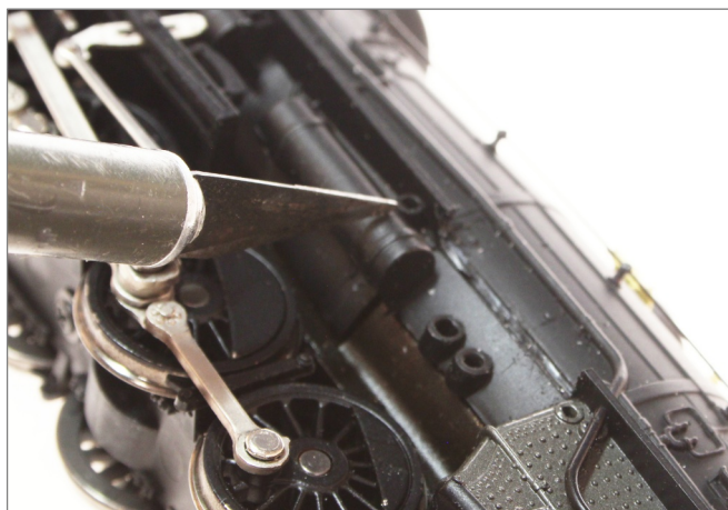
14. The air tank had to be carved away, one sliver at a time, to just under where the knife blade is resting.
