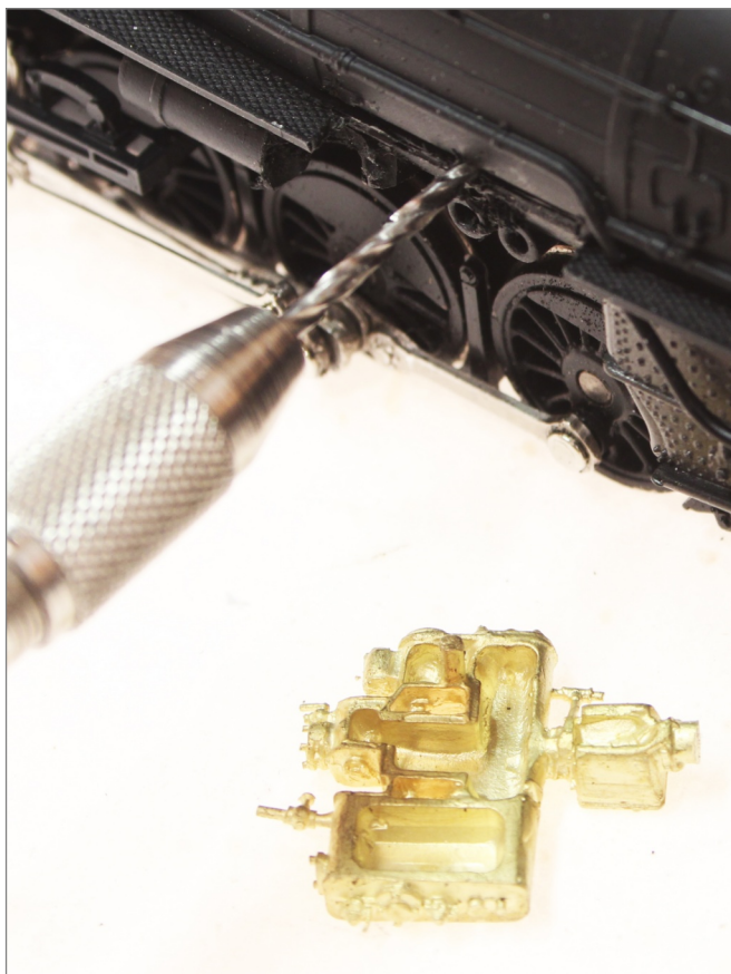
17. Drilling-out the mounting hole for the Worthington feedwater heater.
