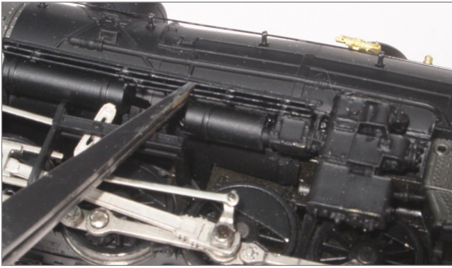
18. Putting the coil pipes back in place.
