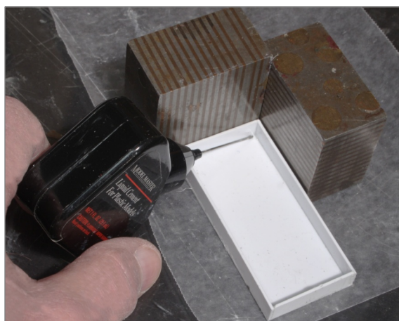
30. I used steel blocks to keep the bunker assembly square and plumb.
