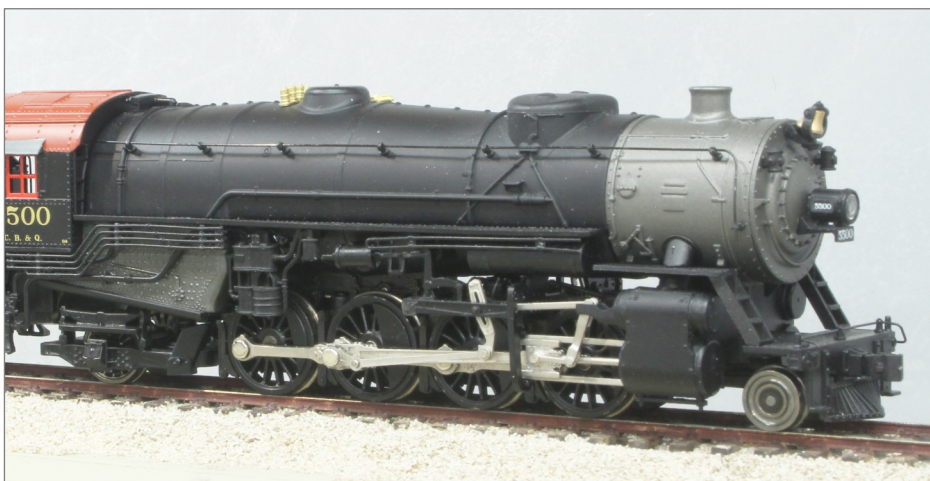
39. An engineer's-side view of the completed USRA Heavy Mikado with its 1920s upgrades. It's a good match to the prototype [1A].
