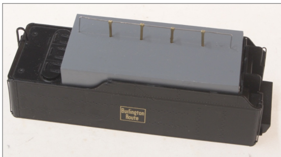
37. The bunker is in place.
