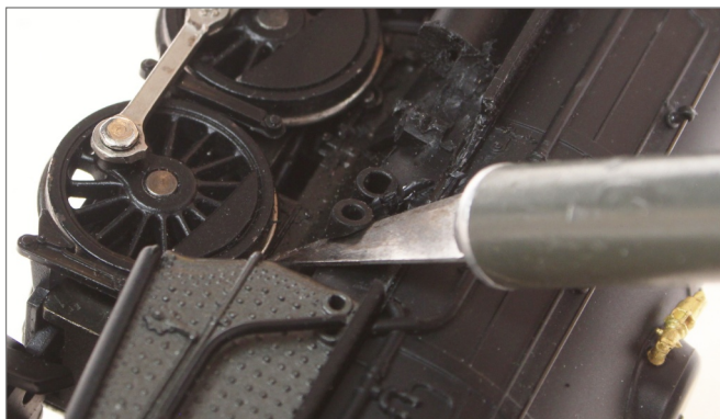
16. Slicing off one of the air pump mounts.
