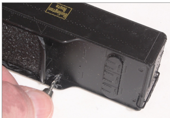
32. Drilling a rear corner for the coal bunker.
