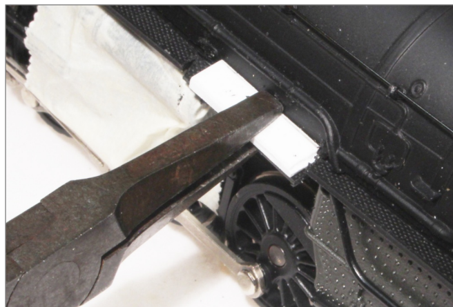
10. I used pliers to break the plastic running board away from the boiler. I covered the top with a scrap of tyrene to protect the molded-on anti-slip grid.
