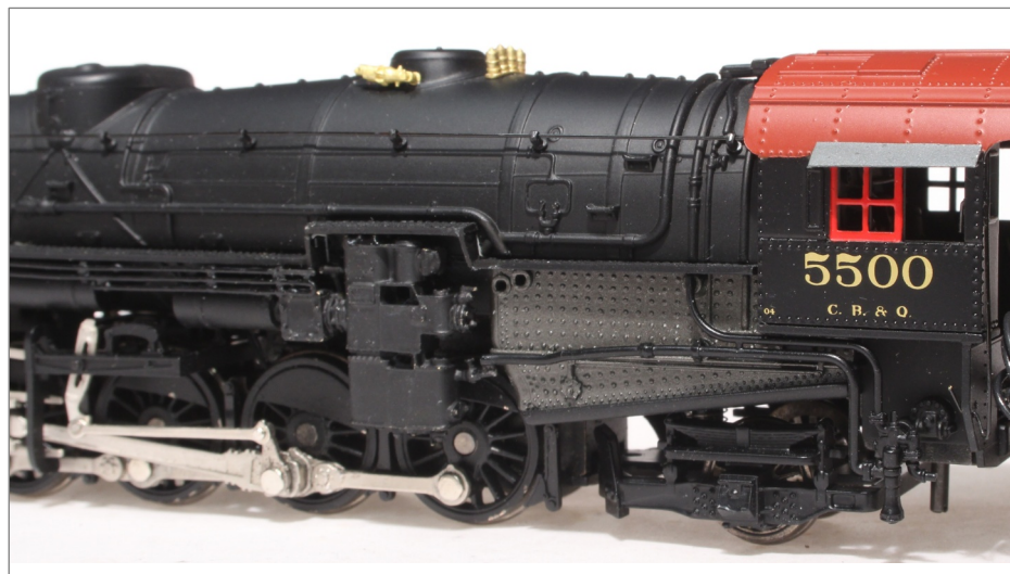
21. The fireman's side modifications are complete, and the Worthington feedwater heater is in place.
