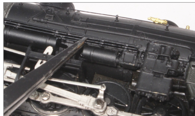
18. Putting the coil pipes back in place.
