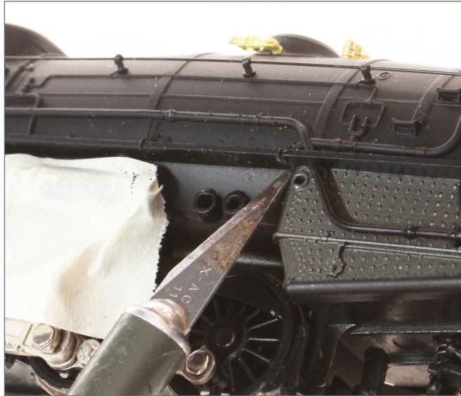
9. Scoring the running board section with the hobby knife created a break line.
