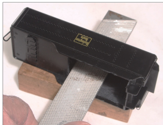
33. I used a file to remove all traces of "coal" from the inside of the coal bunker.
