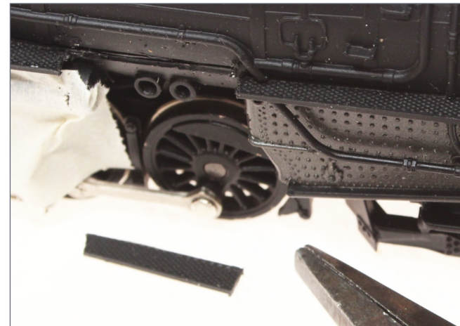
11. With the running board scored, I used pliers to gently flex the cut area of the running board up and down to snap it off the boiler. Then I filed everything smooth.
