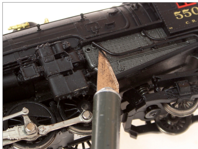
19. Prying the feedwater pipe loose so that it can be bent to align with the feedwater heater.
