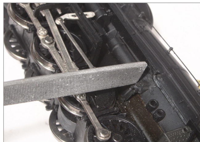
15. Filing the end of the air tank smooth.
