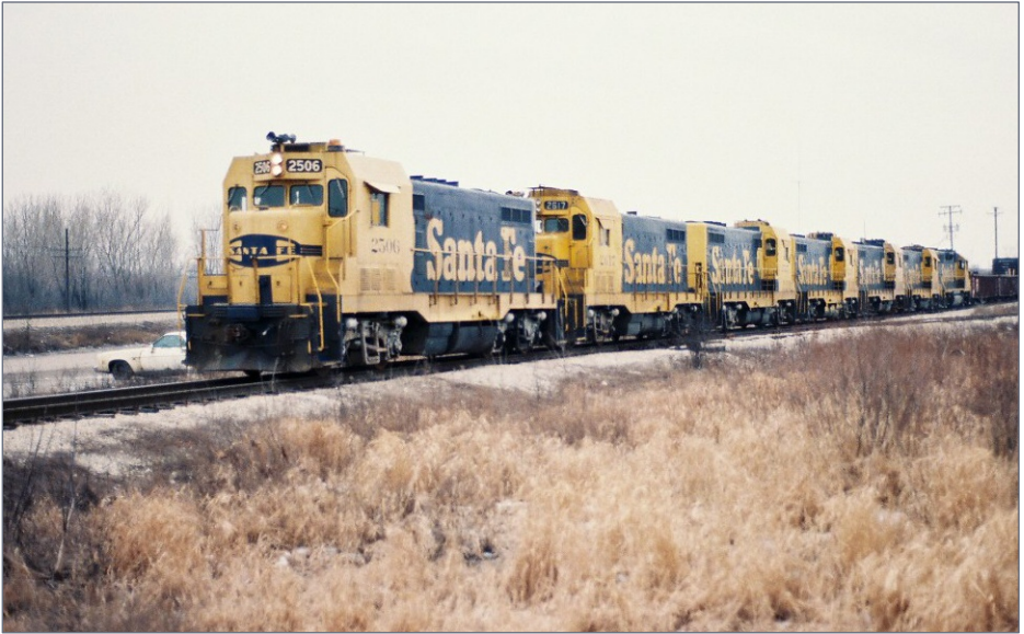
3. Santa Fe CF7 2506 leads five CF7 siblings, with an unidentified EMD unit trailing, at Hodgkins, IL on October 17, 1984. All CF7s have been upgraded with Topeka cabs. Mark Malnekoff photo, RR Picture Archives ( rrpicturearchives.net/pictures/893482 )
