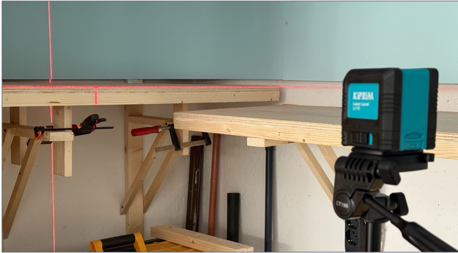
5. A laser level helped me build the layout benchwork perfectly level.
