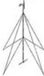
Figure 41: Tower with guy wires
