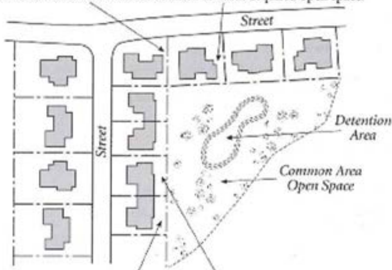
Figure 32: Flexibility with lot sizes and yards can allow for conservation of woodlands and protection of creeks and streams. Detention area not counted towards required open space.
