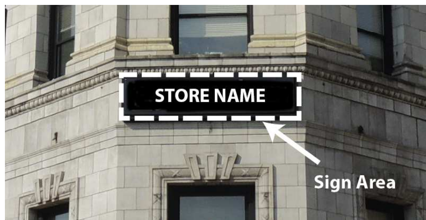
Figure C: Illustration of computing the sign area for wall signs with a background panel or cabinet.
