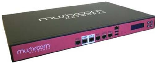
The Truffle™ Broadband Bonding Network Appliance enables an SMB (Small and Medium Sized Business) or an enterprise branch-office (see part II) with faster and more reliable Internet access at an affordable cost by combining various Internet connections into a single IP pipe. The return on investment, compared to alternative single ISP service offerings if available, is often only a few months.
