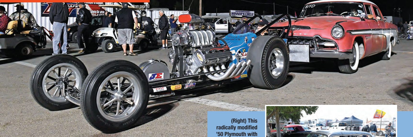
The '61 blown DeSoto-powered B/Fuel Dragster of the Shrank Bros. was push-started appropriately by a '55 DeSoto. The 92-inch wheelbase entry was the 1961 1320 record holder at 8.65, 183.63 mph.
