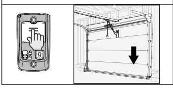
When the door contacts the board, it should stop and reverse direction within 2 seconds to the fully open position. Long LED light on the powerhead will begin to flash RED with the reversal of the door. Remove the 2" x 4" board after a successful contact reversal test. The next cycle will clear the flashing red LEDs.
