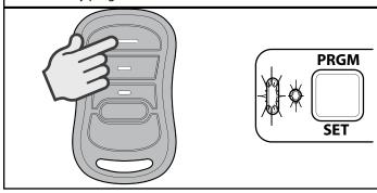
NOTE: While programming remote buttons, stand at least 5 feet away from the powerhead. This ensures you have proper communication between the remote and the powerhead.
