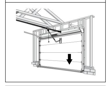
Press and release the program/set button—both LEDs flash blue and then go off.The DOWN (CLOSED) TRAVEL LIMIT IS NOW PROGRAMMED.
