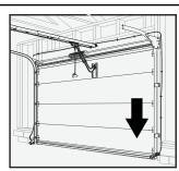
**11.** Press and release the wall console Open/Close button and allow your garage door to travel and stop at the up (open) limit.
