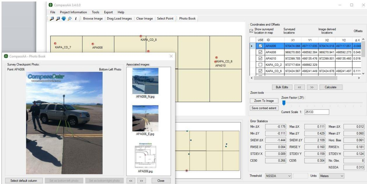
Point 3 (ID column) is an example of a point that is unusable, in this instance because the feature is out of bounds (OB). By clicking on the check mark, the point is unselected and a variety of options of why point is unusable are given. Unused points and the reason selected are displayed in the CompassAA produced report. The list of reasons can be customized by the user in the **Tools ->Options** menu.
