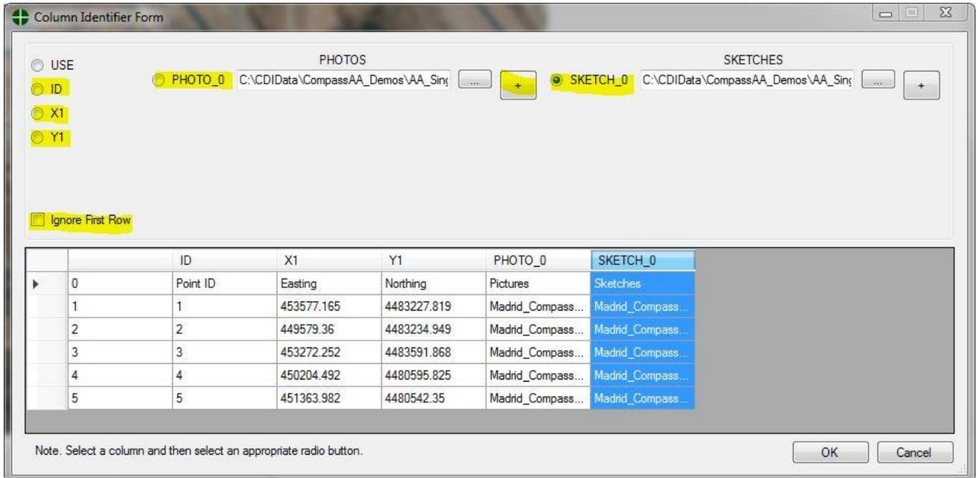
6b. For the Photo and Site Sketch Columns navigate to the **03\_Survey\_Pics** folder or the **04\_Station\_Diagrams** folder. To access multiple photo folders, click on the + button and browse to the proper folder location. For multiple images, all the site photos can be in the same folder but the names need to be similar to the naming convention in the demo. The files must be in .jpg format.
