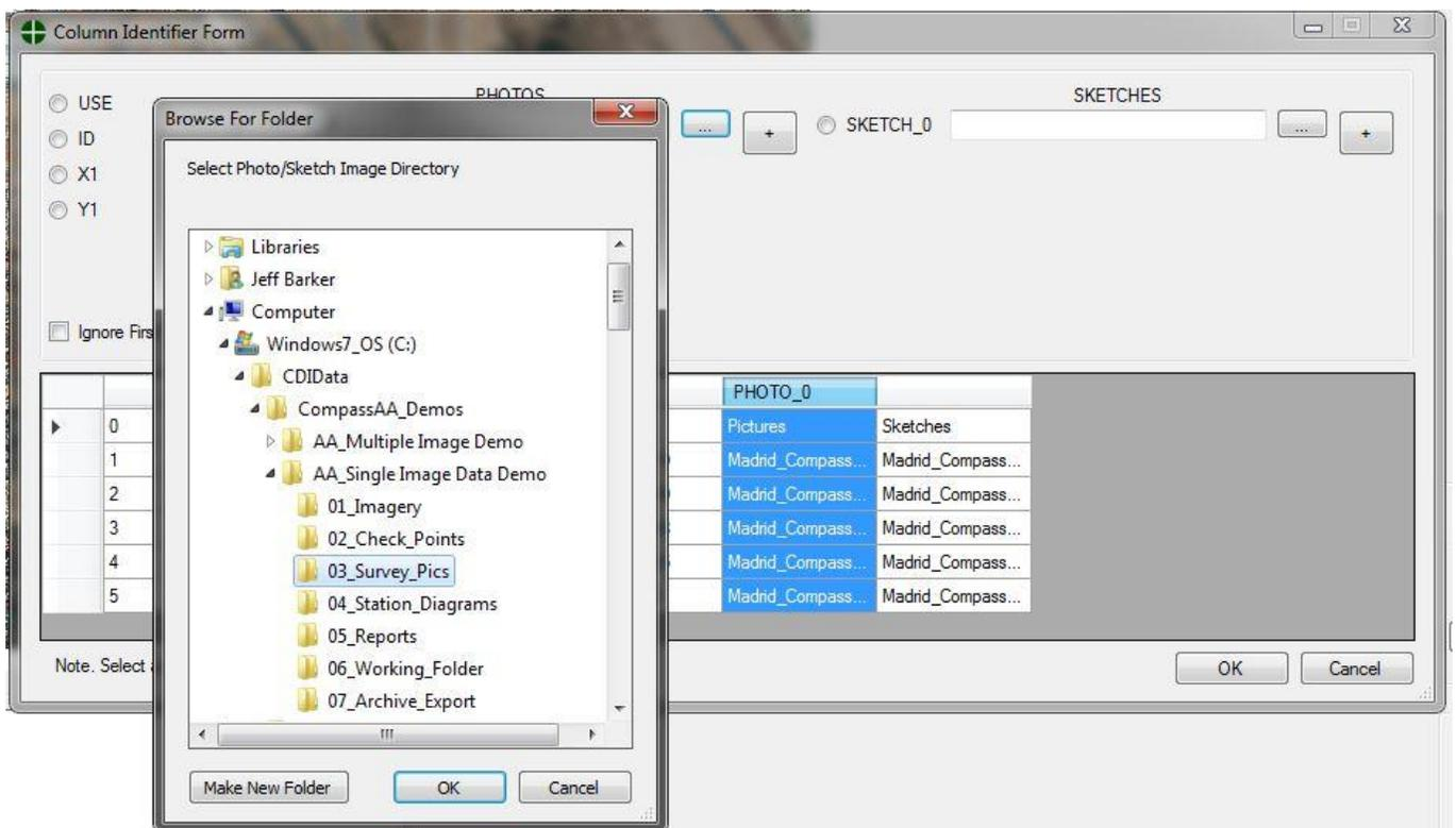
6c. After confirming that the columns of data are selected correctly as in the 6a graphic above, click the Column Identifier Form window **OK** button.
