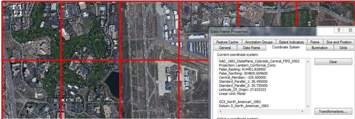
***Note: The image data and checkpoint data must all be in the same map projection with common datum and spheroid. CompassAA does not support automatic projection transformation.***
