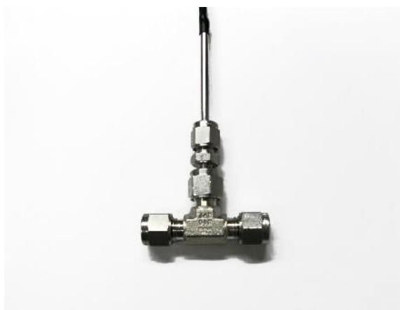
Fig. 5 Dipping probe (top) integrated in Swagelok T-cell (FTCM)
