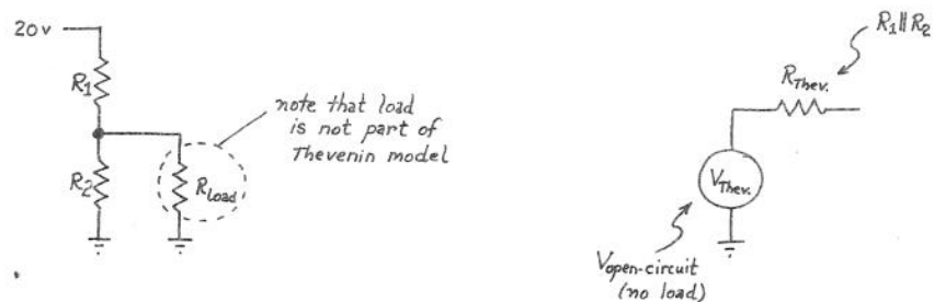
Figure N1.12: Thevenin Model: perfect voltage source in series with output resistance
