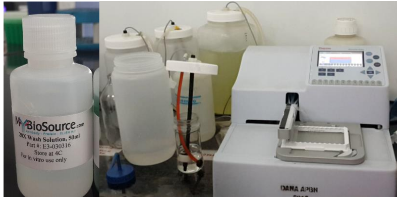
Gambar 6 a. Stok 20x Wash Solution; b. Elisa Washer (Thermo Scientific™ Wellwash™ Microplate Washer)
