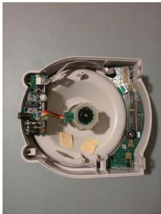
Once it's apart you'll see two circuit boards at opposite ends of the unit and a motor in the middle. The motor is well padded with soft plastic that you shouldn't touch with oily fingers. You'll see a tachometer attachment on the bottom of the motor and 5-wire connector that attaches to the circuit board at the back of the unit. It can be disconnected from this unit and the motor *carefully* set aside. The two circuit boards are held on with screws and padded with double sided foam tape.
