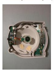
Once it's apart you'll see two circuit boards at opposite ends of the unit and a motor in the middle. The motor is well padded with soft plastic that you shouldn't touch with oily fingers. You'll see a tachometer attachment on the bottom of the motor and 5-wire connector that attaches to the circuit board at the back of the unit. It can be disconnected from this unit and the motor *carefully* set aside. The two circuit boards are held on with screws and padded with double sided foam tape.
