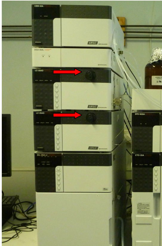
Figure 4: Turn black wheels on Pump A and Pump B 90° to the left
