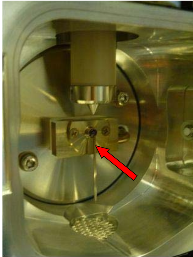
Figure 1: Plug in ion inlet of mass spec
