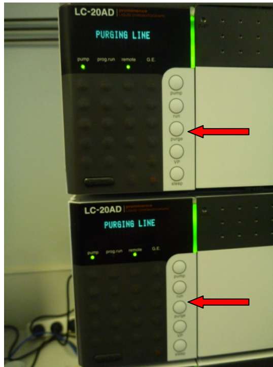
• Figure 6: Press purge on Pump A and Pump B
