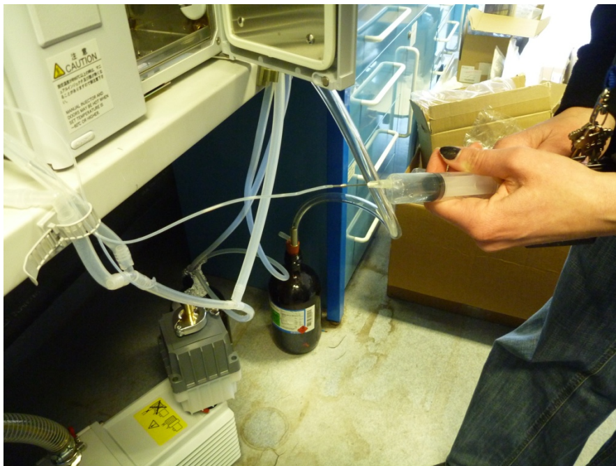
Figure 5: Syringe out 10-15 mL solvent from line A and line B
