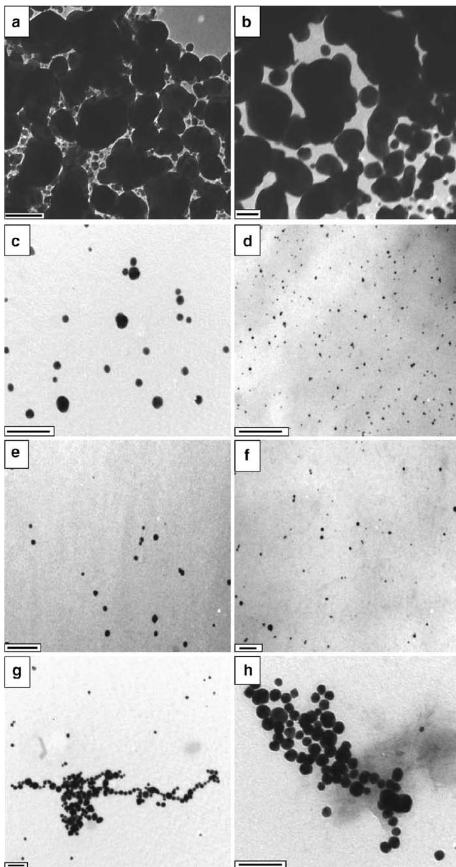
**Fig. 2.** TEM images of blank gold nanoparticles reduced using varying concentrations of chitosan **a** 0.01% w/v, **b** 0.05% w/v, **c** 0.1% w/v, **d** 0.2% w/v, **e** 0.5% w/v and **f** 1% w/v, and insulin loaded gold nanoparticles reduced using 0.2% w/v chitosan **g** and **h**.
