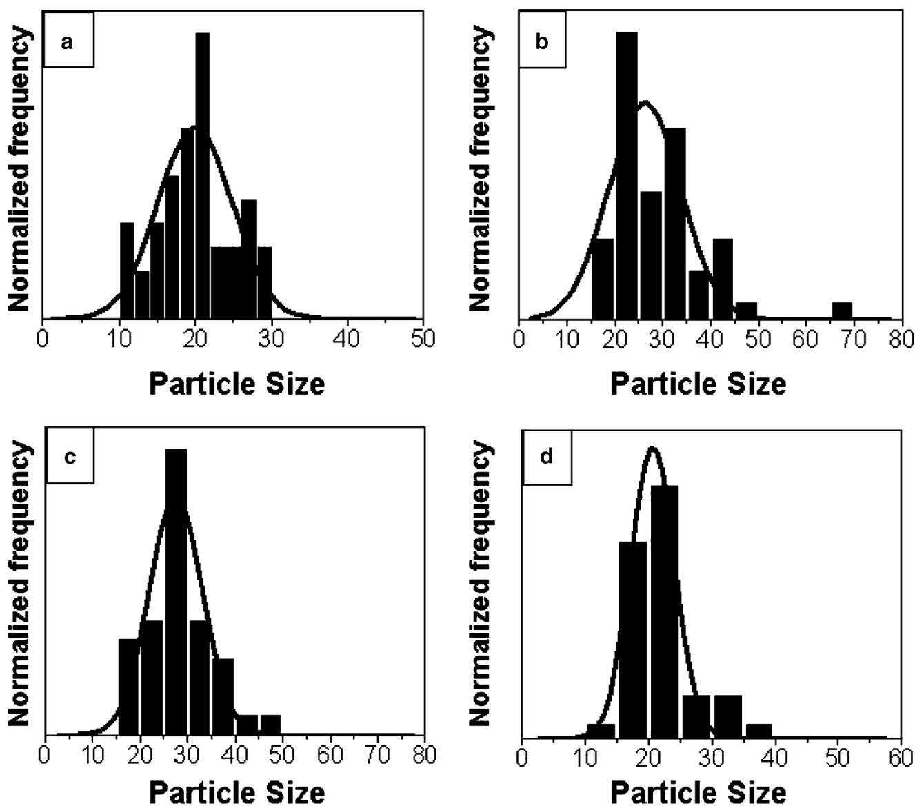
Fig. 5. Particle size distribution of gold nanoparticles synthesized using varying concentrations of chitosan **a** 0.1% w/v **b** 0.2% w/v **c** 0.5% w/v **d** 1% w/v.
