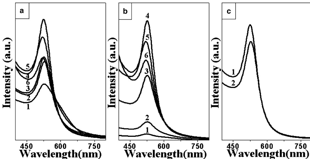
**Fig. 3.** Visible absorption spectra of gold nanoparticles synthesized using varying concentrations of chitosan **a**  $t=0$ ; **b**  $t=6$  months, where curve (1) 0.01% w/v, (2) 0.05% w/v, (3) 0.1% w/v, (4) 0.2% w/v, (5) 0.5% w/v, (6) 1% w/v. **c** Visible absorption spectra recorded from the chitosan (0.2% w/v) reduced gold nanoparticle dispersion before (curve 1) and after loading with insulin (curve 2).
