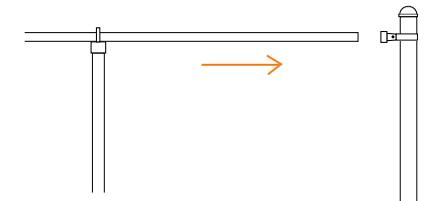
Continue to feed additional top rails through line post caps. Connect rails by inserting tapered end of rail into next rail.
