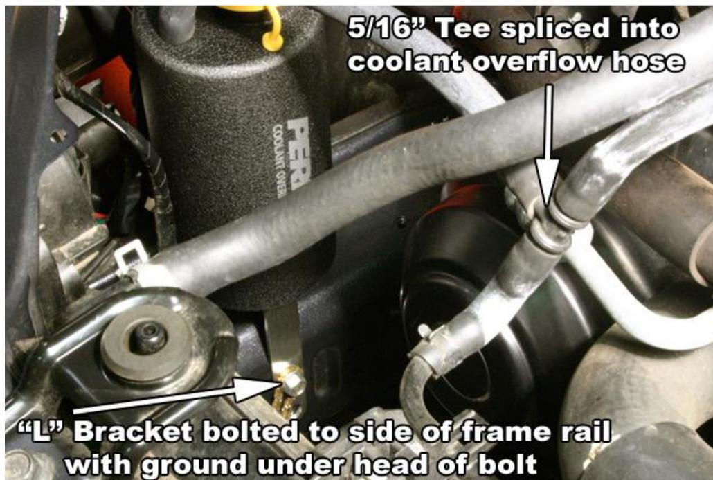
6. Push supplied 5/16" silicone hose into medium size hole on top of tank. Push hose through hole until it hits the bottom of tank. Pull hose out roughly .5" so hose doesn't touch bottom of tank.
