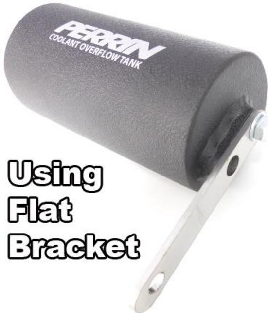
4. Using Supplied M8 Bolt and washer, bolt flat 3 hole bracket to one of (2) holes on bottom of coolant tank. We recommend the centered hole as this will provide the best fit on most cars. The other hole can be used in cases where different intercoolers are used or other aftermarket parts are installed.
