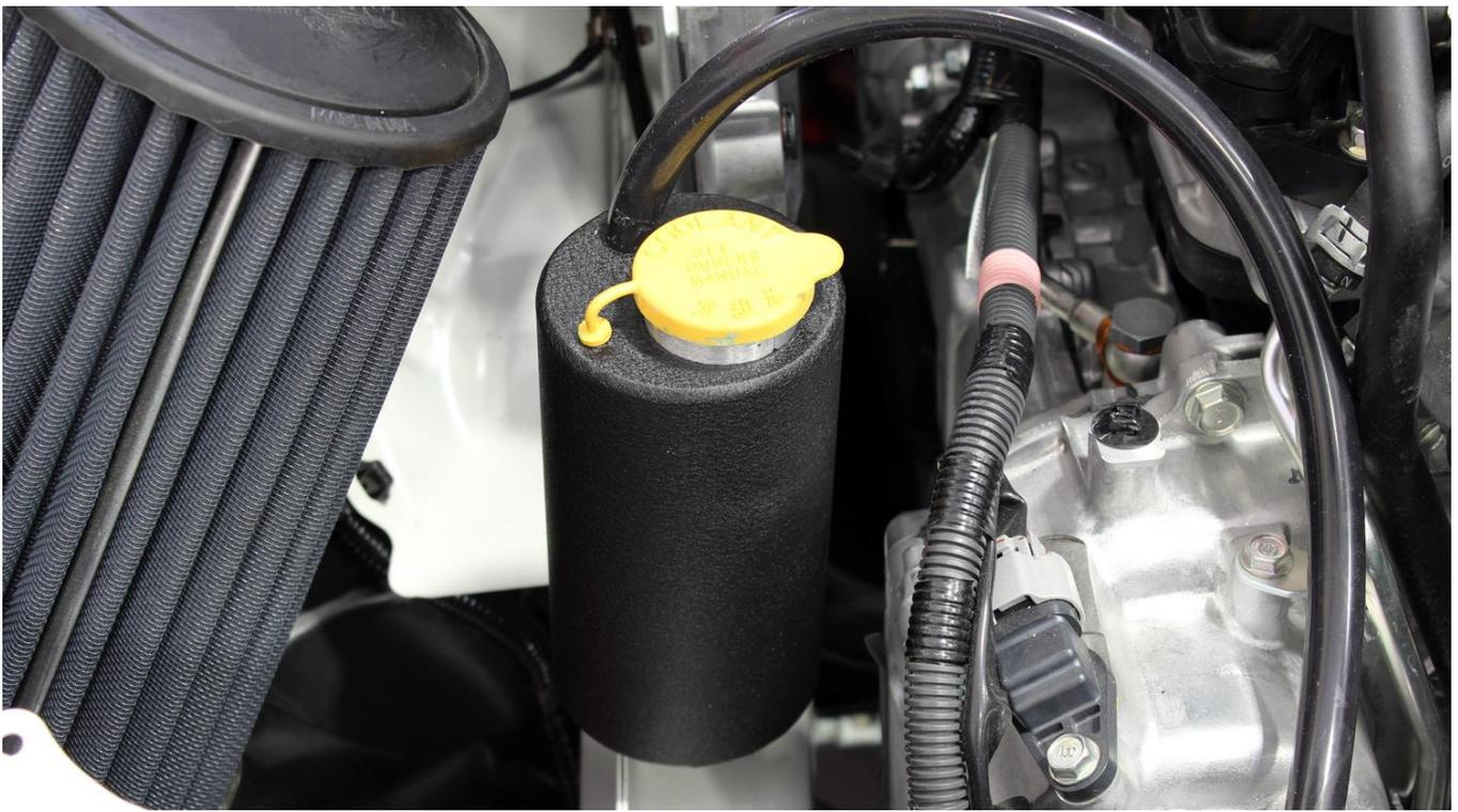
8. Snap cap onto PERRIN Coolant Overflow Tank and push barbed end into remaining small hole on top of can.
